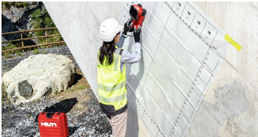
a) Scanning for ferrous objects
