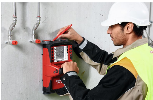
c) Scanning for ferrous &amp; non-ferrous objects
