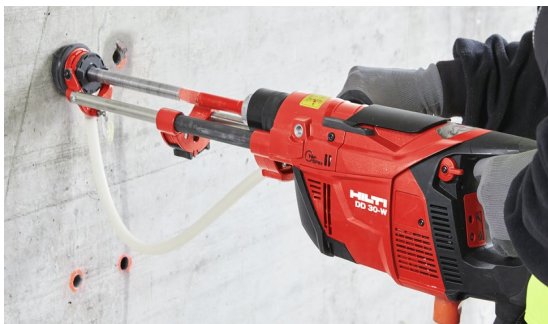
a) Diamond core drilling (Hilti DD 30-W)
