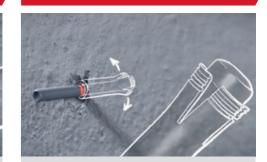
Undercut anchors are a favorite for engineers because of their safe and reliable mechanical interlock.
