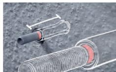
The red setting indicator mark is exposed when the sleeve has moved down
