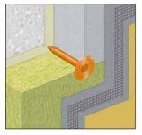
The XI-FV fastener is used to transfer wind suction loads acting on the thermal insulation composite system.
