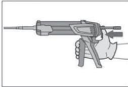
Inject the mortar from the back of the hole towards the front and slowly withdraw the mixing nozzle step by step after each trigger pull.
