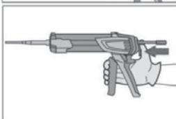
Insert piston plug to back of the hole. Begin injection allowing the pressure of the injected adhesive mortar to push the piston plug towards the front of the hole.
