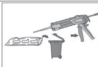
Discard initial mortar. The foil pack opens automatically as dispensing is initiated. Depending on the size of the foil pack an initial amount of adhesive has to be discarded.
