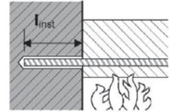
Maximum force in rebar in conjunction with HIT-RE 500 as a function of embedment depth for the fire resistance classes F30 to F180 (yield strength  $f_{yk} = 500 \text{ N/mm}^2$ ) according EC2<sup>a)</sup>.
