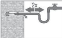
In addition for wet diamond coring (DD):
