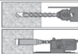
Drill the hole to the required embedment depth using a hammer-drill with carbide drill bit set in rotation hammer mode, a compressed air drill or a diamond core machine.
