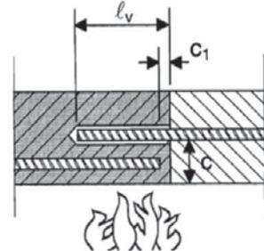
Critical temperature-dependent bond stress,  $\tau_c$ , concerning “overlap joint” for Hilti HIT-RE 500 injection adhesive in relation to fire resistance class and required minimum concrete coverage  $c$ .
